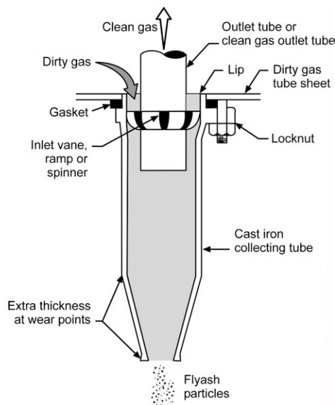
Figure 2-8. Cyclone tube used in multi-cyclone collector
