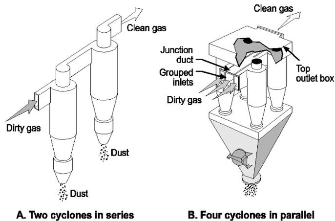
Figure 2-5. Series and parallel arrangement of cyclones
