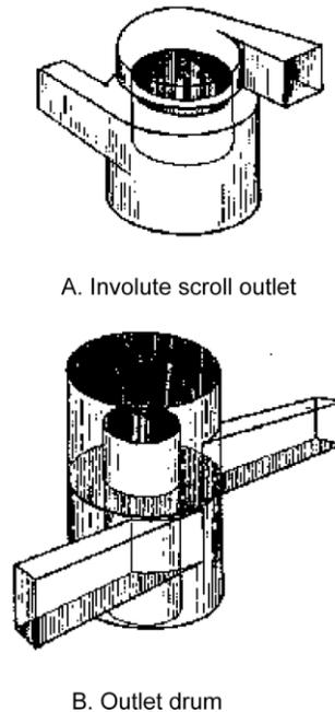
Figure 2-4. Special outlet configuration for large diameter cyclones
