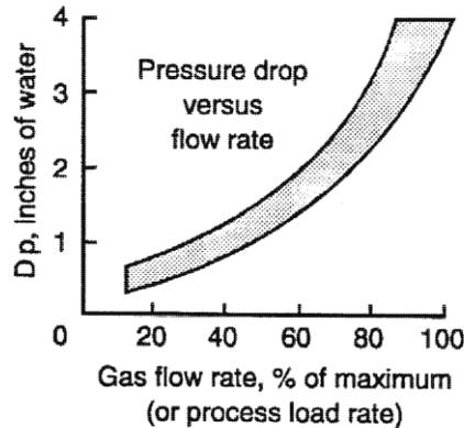
Figure 2-10. Static pressure drop of a cyclone collector
