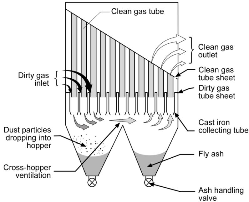
Figure 2-9. Cross hopper recirculation
